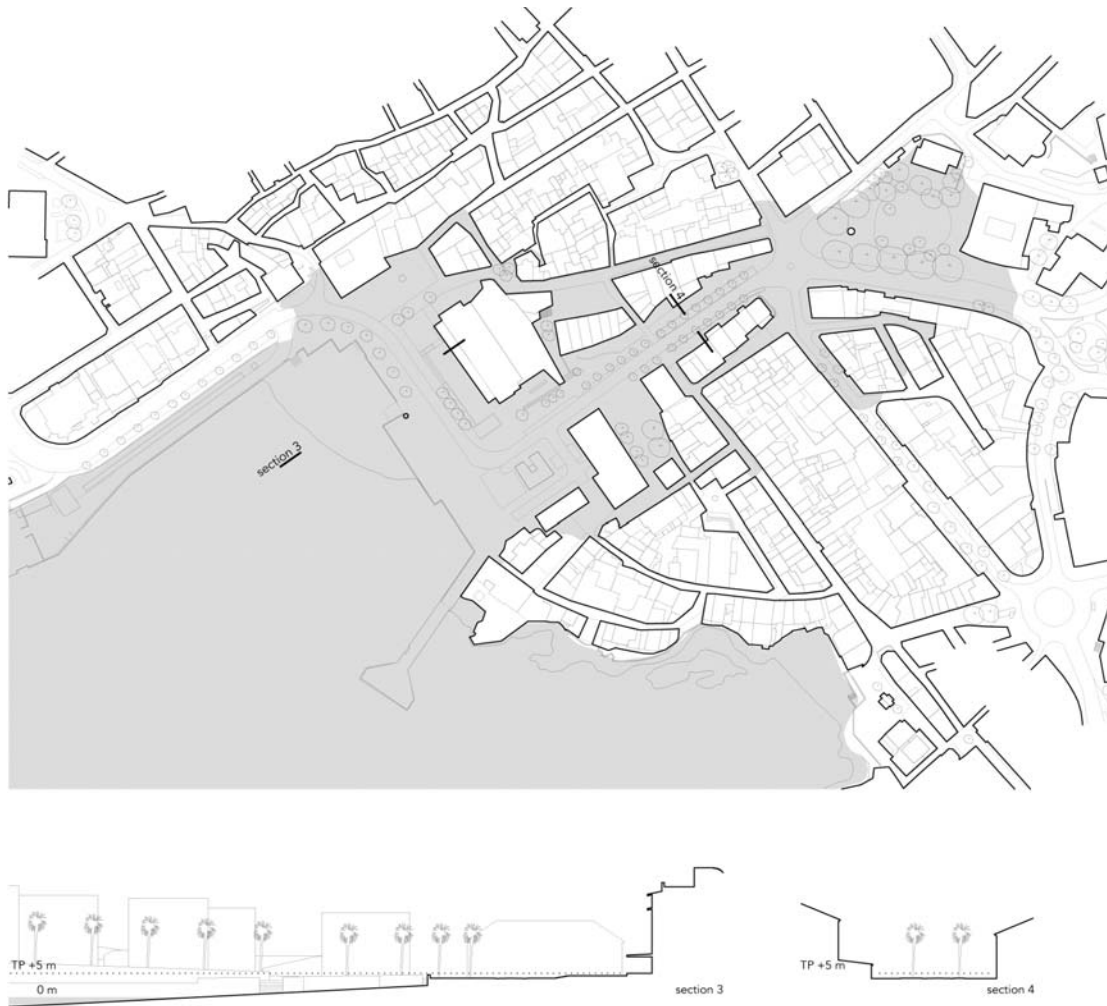
Figure 7: Cascais seashore street. Detail plan (rotated 90° clockwise) and cross sections considering a +5m sea level rise. Source: (Forma Urbis Lab and Author)
