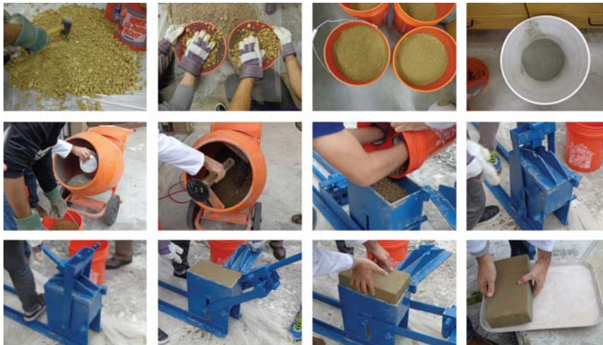
Figure 3: Multi-step compressed stabilized earth block fabrication process. Source: (Author)
