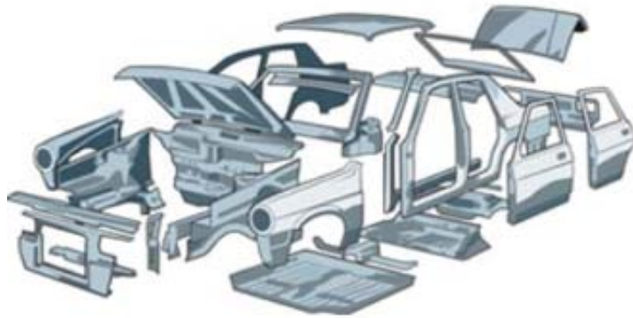
Figure 2: Car Stamping Diagram Source: (USA 2009)
