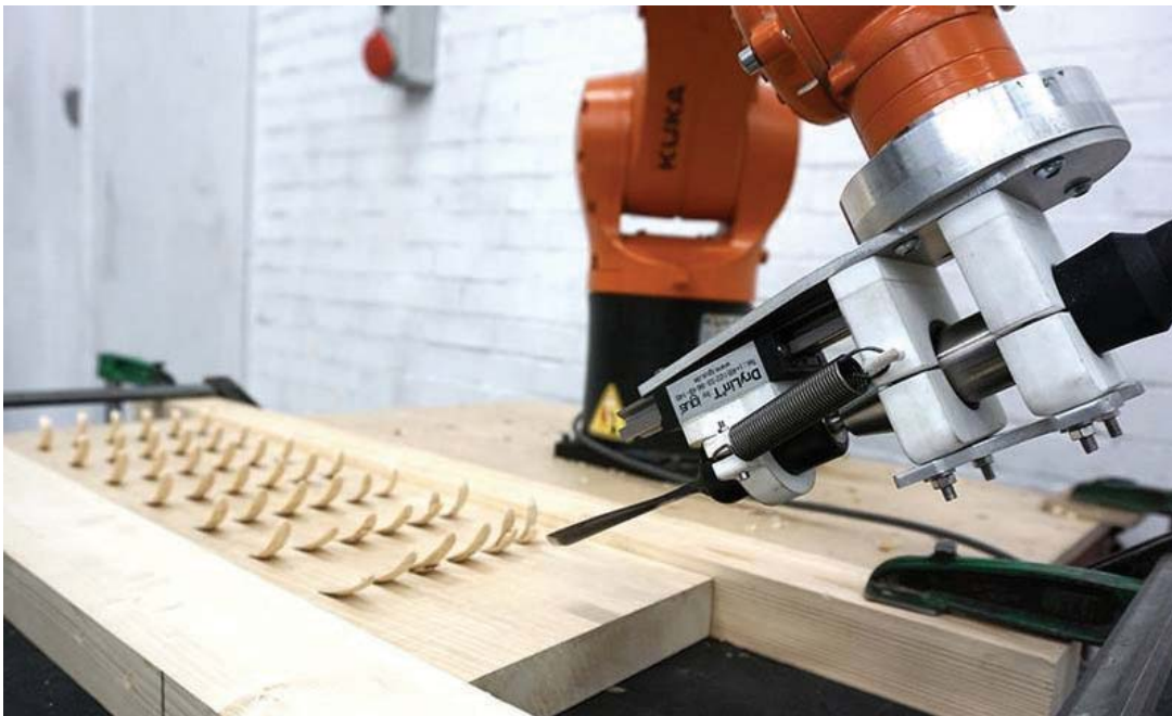
Figure 1: Innochain: Adaptive Robotic Carving. Source: (Giulio Brugnaro)
