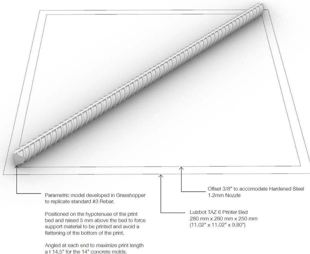
*3D printed rebar, modeled and oriented for TAZ 6 printer bed.*
