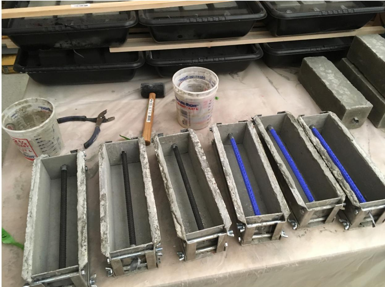
*Concrete molds with carbon fiber PLA (left) and ABS (right) rebar.*
