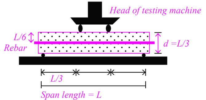
Diagram of testing set up.
