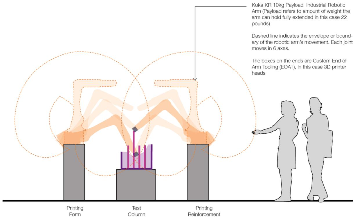
*Proposed workcell configuration for multi-material formwork printing.*
