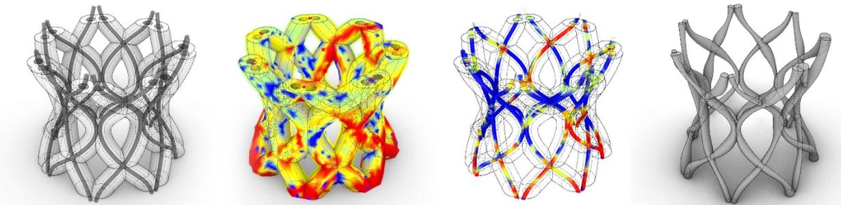
*Karamba analysis of concrete column, illustrating transfer of forces to variable-profile reinforcement model*
