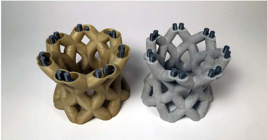
*Polyvinyl Alcohol (PVA) formwork with Steel PLA reinforcement*
