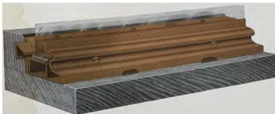
Figure 2 “Metal Sash No. 30.” One of Kawneer’s first products was a copper clamping system that formed a sash around storefront windows. Source: Kawneer Store Fronts , 1912.
