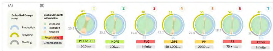
Figure 1: Thermoplastic Profile Medallions: Showing (A) Embodied Energy of production, recycling, and molding processes as well as (B) global circulation ratios of annual production, recycling, and disposal with recyclability levels, and decomposition estimations. Source: Content pertaining to diagram was sourced from (Ashby 2013).
