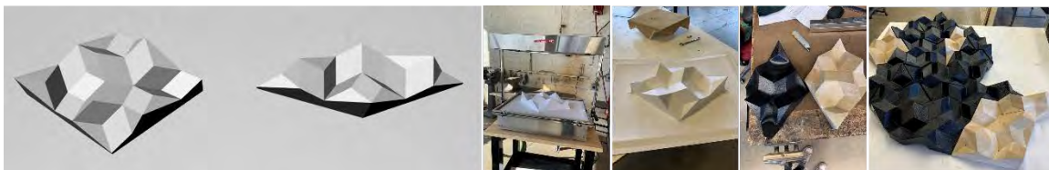
Figure 11: Vacuum forming of two quasi-periodic surface units (school of architecture, University of Utah). Source: (Ajlouni & Feltovich 2021).
