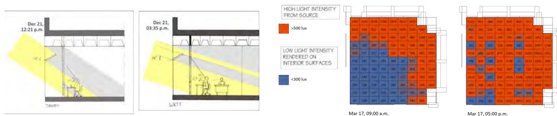
Figure 8: Challenges of the daylighting situation in the space, daylight glare presence due to the variations in windows' luminance values at sunny portions versus shaded portions (first and second images from left), under-illuminated areas <300 lux (third image from left), and over-illuminated areas >500 lux (last image on the right). Source: authors.
