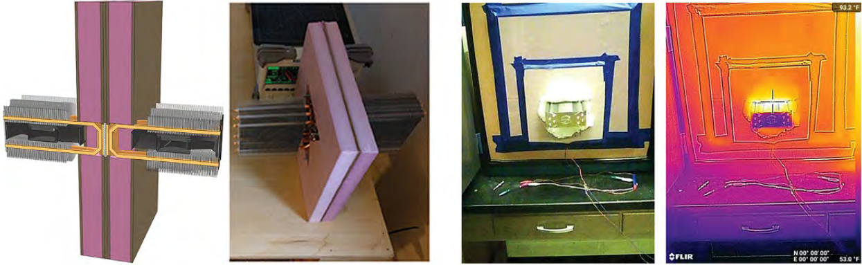
Figure 1: Experimental prototype and thermal imaging. Source: (Author 2018)
