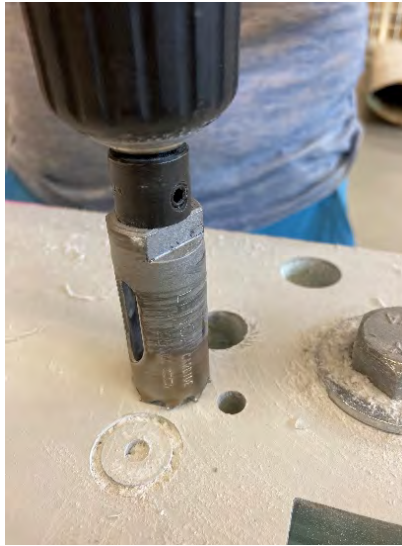
Figure 13: Drilling of hardware holes with diamond saw
