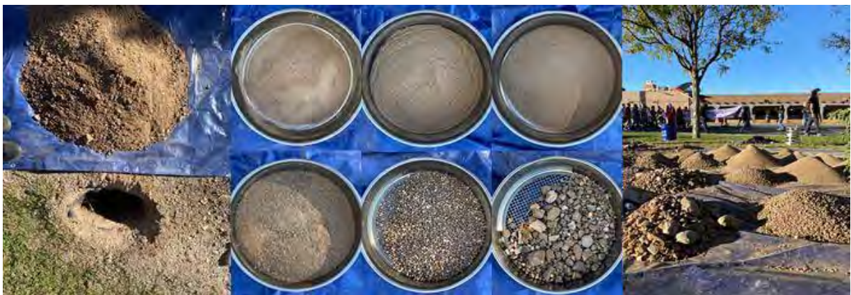
Figure 4: On-site soil particle analysis. Source: (Authors 2021)
