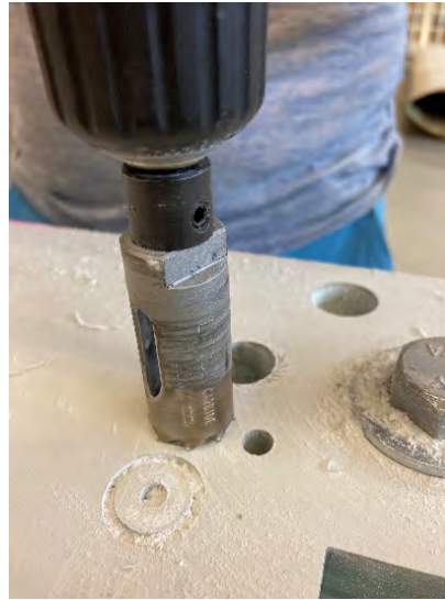
Figure 13: Drilling of hardware holes with diamond saw
