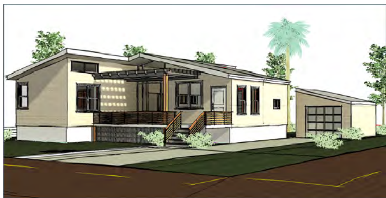
Figure 4: Core+ view adding a breezeway inbetween the units with other design modifications after years of unit installation and adapting by means of AMHD design capacity resulted from the community workshop. Source: (Author 2021)
