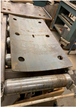
Figure 10: Steel is formed to fit blade curvature
