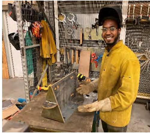
Figure 11: Steel plates are CNC waterjet cut and MIG welded to create the final UC
