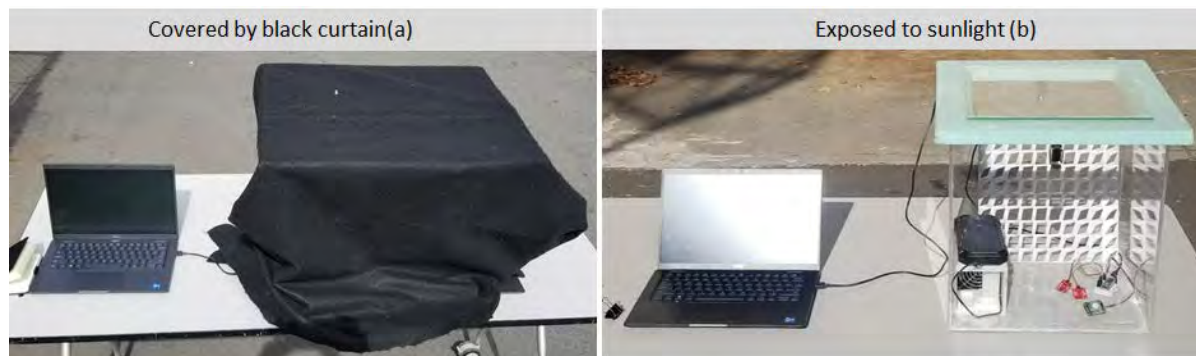
Figure 5: TiO 2 photocatalytic facade testing setup
