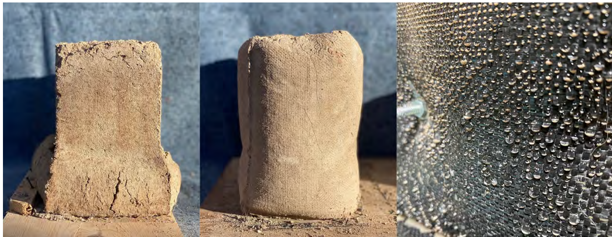
Figure 6: Side by side comparison of standard wood formwork (left, with resultant slumping) and fabric formwork (center, no slumping because of even drying). Forms removed after two weeks. Detail of water escaping fabric at right. (Source: Authors 2021)
