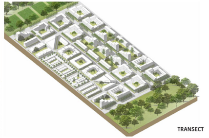
Figure 7. An exploration of blue-green infrastructure broken down by neighborhood level to help offset the seasonal flooding in Mexico City and to help alleviate land sinking issues as a result of underground water depletion. Source: (Gayatri Tawari 2016)
