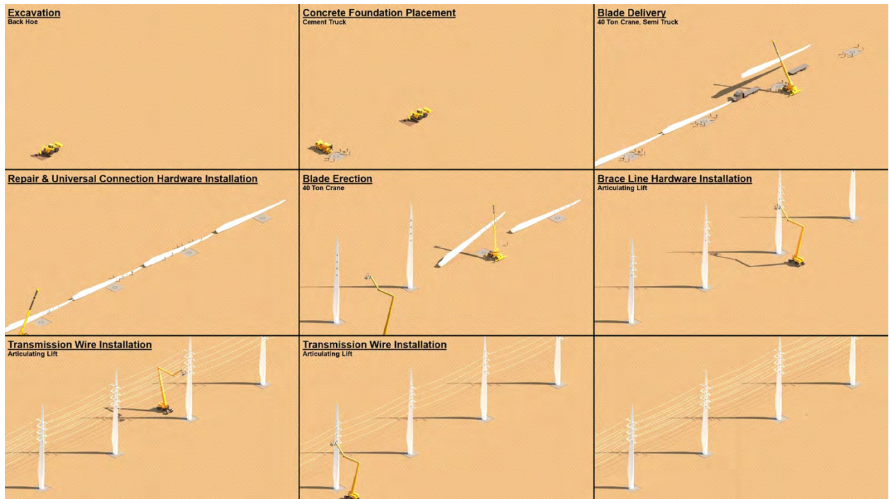
Figure 7: BladePole construction sequence in the field: 1) Excavation of site, 2) Concrete foundations are placed, 3) Blades are delivered, 4) Blade repairs are made and UC's are installed, 5) Blade erection with small crane, 6) Braced Line Post Hardware is installed, 7) Transmission wires are installed on first side, 8) Transmission wires are installed opposite side
