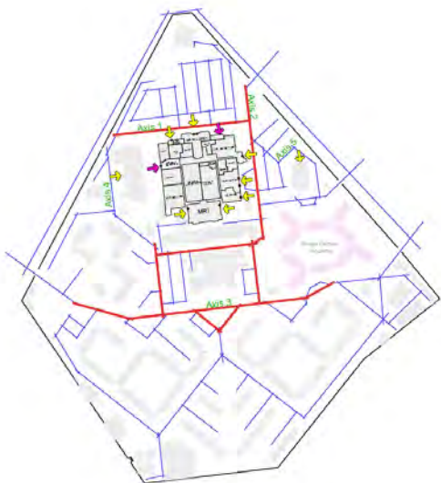
Figure 11: The syntactic analysis of vehicular system of the KFSH campus showing the integration core at radius 'n' (10% of all the axes)
