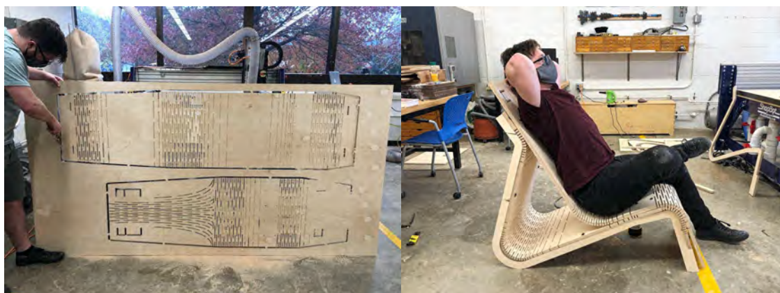
Fig. 2a & b Kerf Bent Chair by Nicolas Di Donato and Hana Saifullah. (a) Plywood sheet routed with pattern before bending. (b) Final chair.
