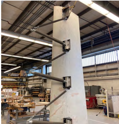
Figure 15: UC and Braced Line Post hardware is completely installed and blade is erected in the lab awaiting a full-scale structural test
