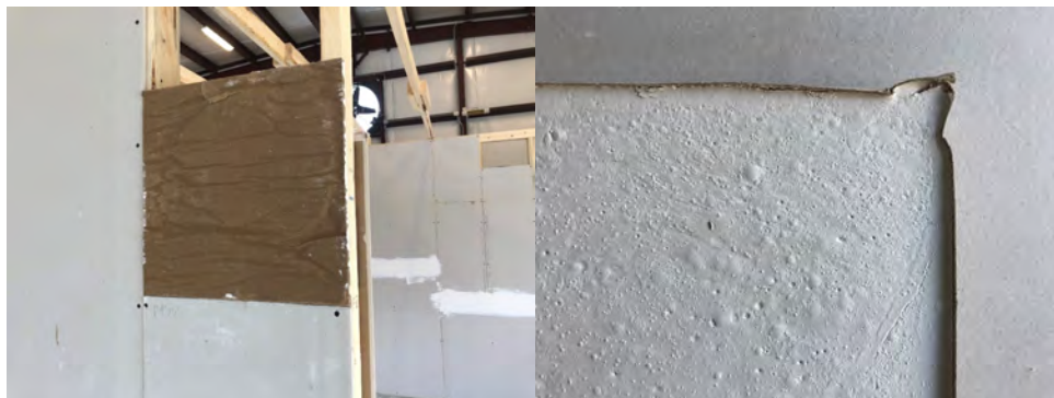
Figure 2: Cast gypsum wallboard panels demonstrated method for small scale fabrication. Source: (Author 2021)
