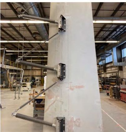
Figure 14: UC and Braced Line Post hardware is completely installed and blade is erected in the lab awaiting a full-scale structural test
