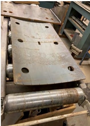
Figure 10: Steel is formed to fit blade curvature
