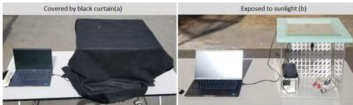
Figure 5: TiO 2 photocatalytic facade testing setup
