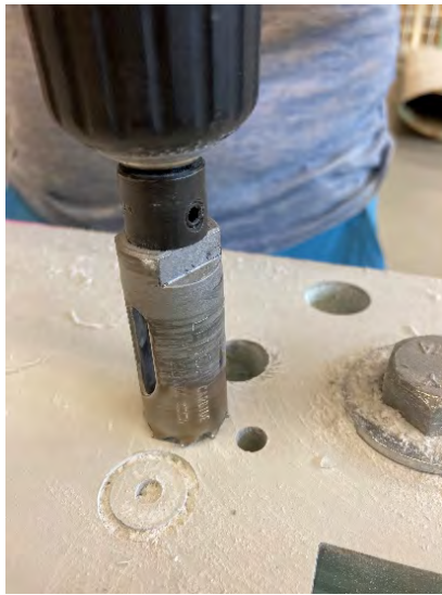
Figure 13: Drilling of hardware holes with diamond saw
