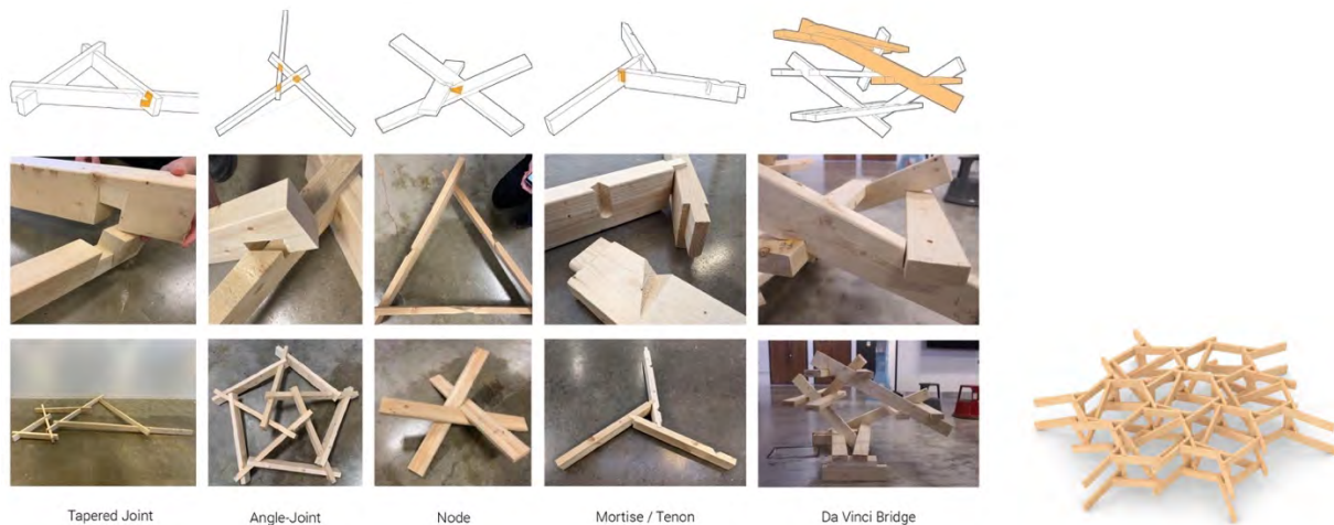
Fig. 3. Jointing conditions of reciprocal frame nodes and an example of a double layer reciprocal frame with interstitial members in between as a type of 3D truss frame.
