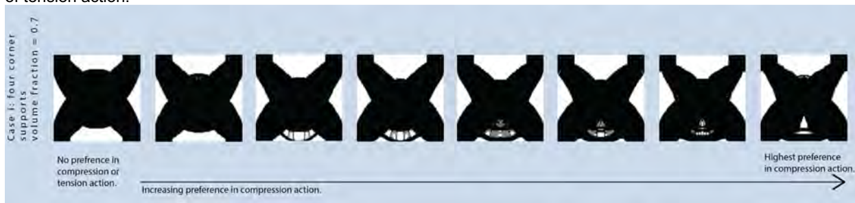
Figure 5. Case i with 0.7 volume fraction can have many shapes based on a change in the preference in the amount of compression action.
