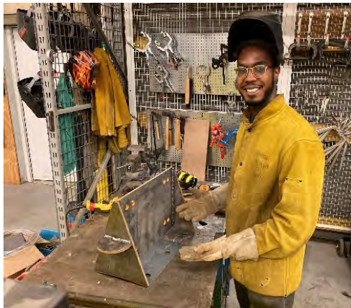
Figure 11: Steel plates are CNC waterjet cut and MIG welded to create the final UC
