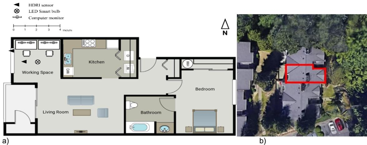
**Figure 1:** Example of home-office layout. a) plan shows where the subjects were seated, positions of computer monitors, LED smart bulb, and locations and view orientations of HDR1 sensors, b) surrounding urban context.
