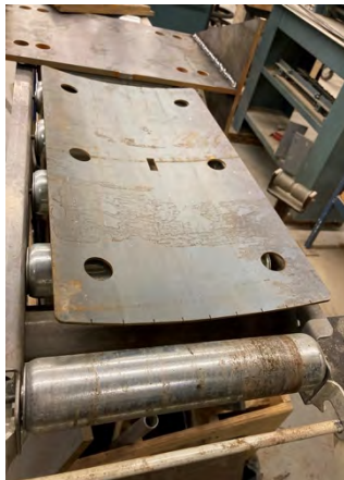
Figure 10: Steel is formed to fit blade curvature
