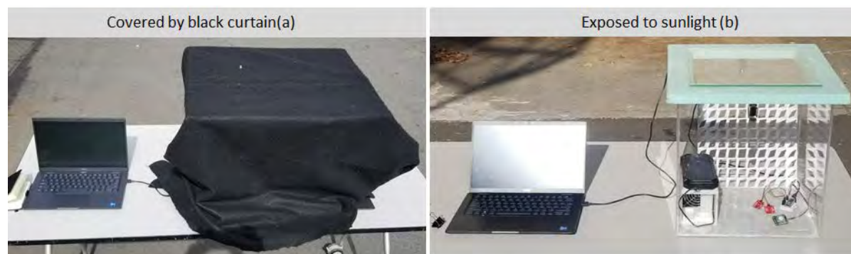
Figure 5: TiO 2 photocatalytic facade testing setup
