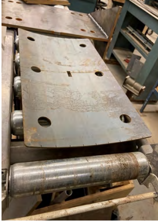
Figure 10: Steel is formed to fit blade curvature
