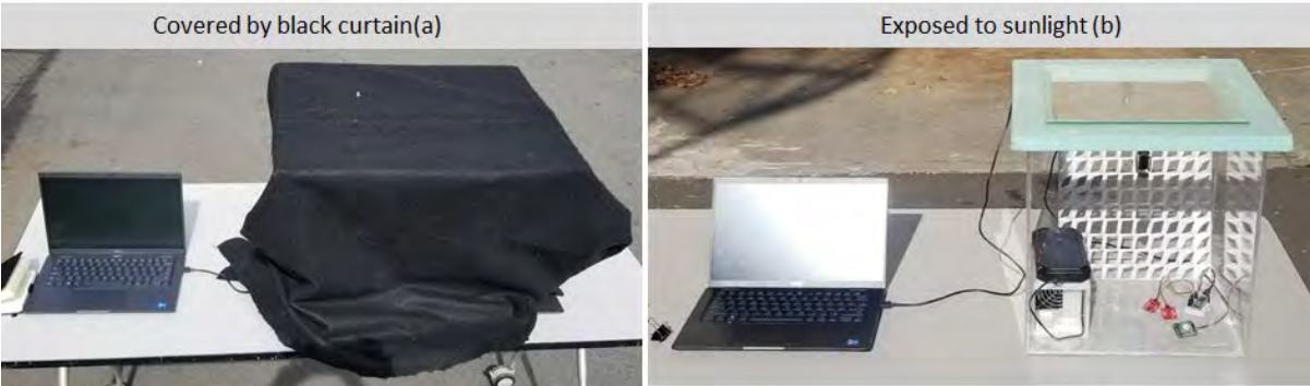
Figure 5: TiO 2 photocatalytic facade testing setup
