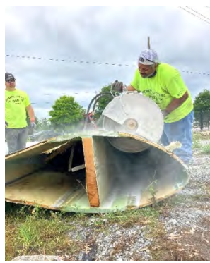
Figure 9: Large sections are cut into smaller test specimen
